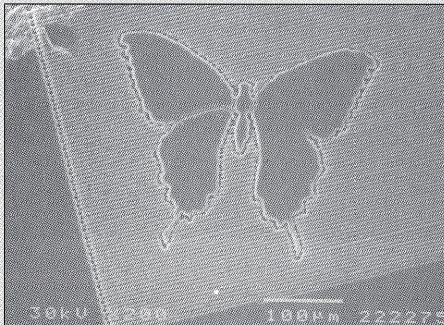
Figure 4. Butterfly formed in relief in a polished diamond surface. Overall width of the structure is 300 \mu\text{m} .
